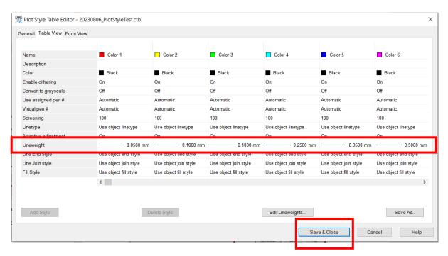
In your drawing model space apply these colours to your layers via the Layer Properties window. And ensure each object has its set to ByLayer. You may need to select all the objects in a layer then change this colour setting.
