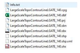
10. Shapefiles/Geopackages cannot be opened directly into standard AutoCAD. One of the simplest (free) methods to convert shapefiles to dxf (which opens in AutoCAD) is using QGIS. Download and install the latest long term release version of QGIS from here: <a href="https://www.qgis.org/en/site/forusers/download.html">https://www.qgis.org/en/site/forusers/download.html</a>. Accept all the installation defaults.
