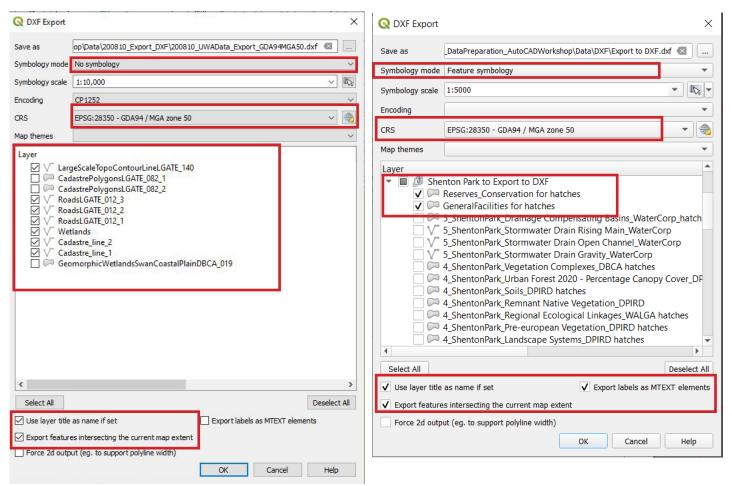
3. This output dxf can be opened in AutoCAD. The layers can be copied to the other drawing containing the Nearmap image using COPYBASE. If you use COPYBASE (not any other copy) and specify the base point as (0,0,0) then PASTECLIP to (0,0,0) in the other drawing, the data will overlay correctly with the Nearmap image. Do not manually move any data.
