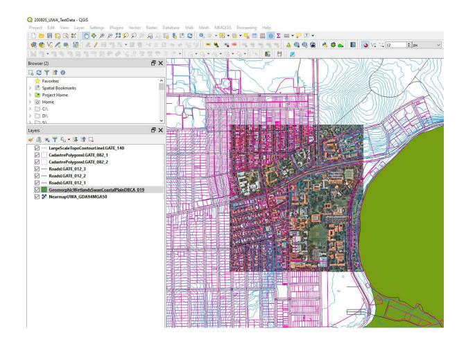
15. When converted to dxf, polygon shapefiles open as hatched areas. It can be more useful to have closed polyline data for AutoCAD. To achieve this, convert the polygon shapefiles/geopackages to line shapefiles before exporting to dxf. First click on the Toolbox "cog" to open the Processing Toolbox window. Then search for Polygons to Lines. Double click to open the tool.
